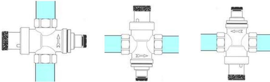
All pressure reducers are tested before being packed; during the test they are calibrated in output at a pressure of 3 bar; the outlet pressure can be easily changed once the reducer is installed on the system.
